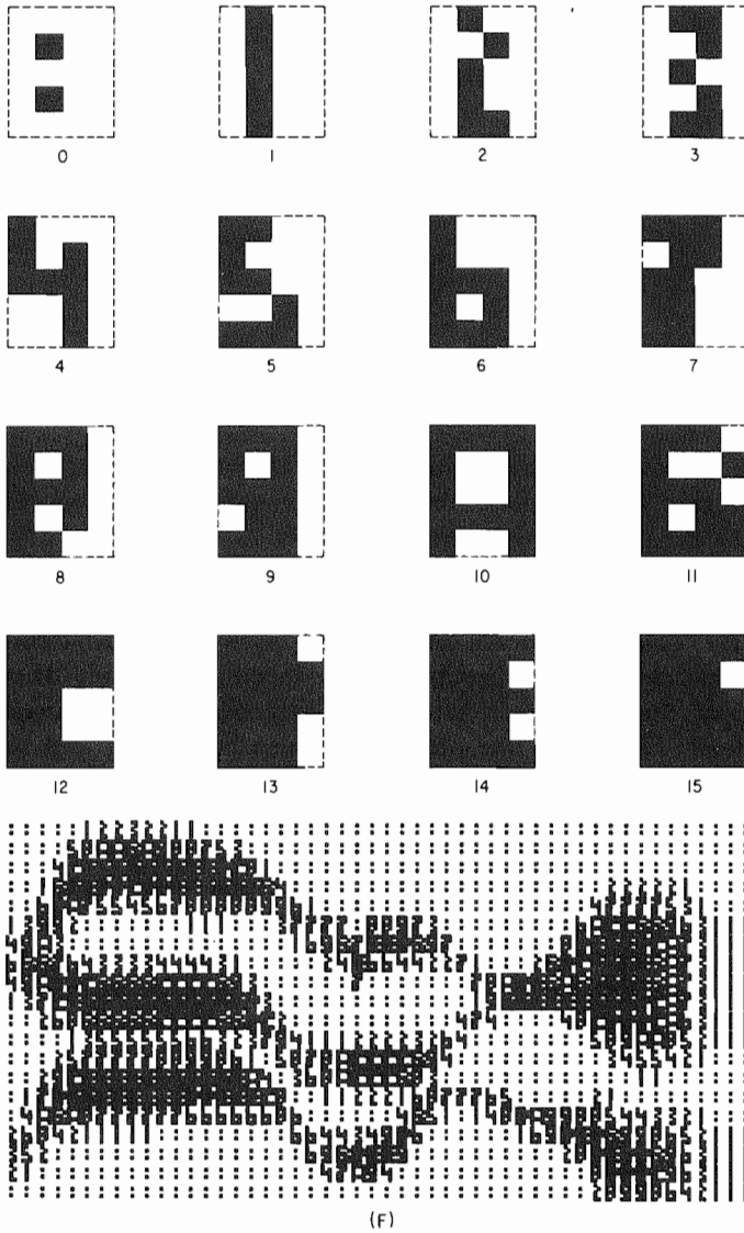
Fig. 16-1. Methods of representing three-dimensional spectral data in two dimensions ( cont. ). (F) Optically weighted character set. Spectral plot using optically weighted characters.
