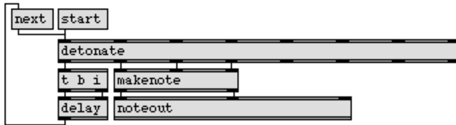
The delta time of the next note is used as the delay time before triggering the next note
