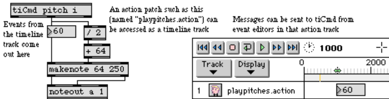
A timeline communicates with an action patch via the ticmd object
