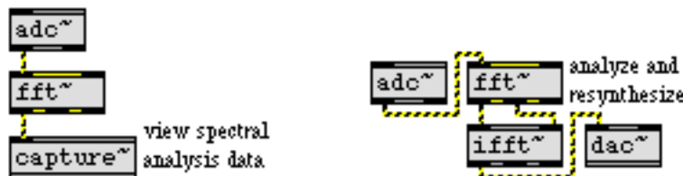
Fast Fourier transform of an audio signal
