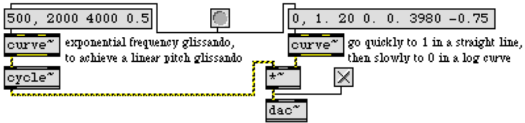
Curved ramps used as control signals for frequency and amplitude
