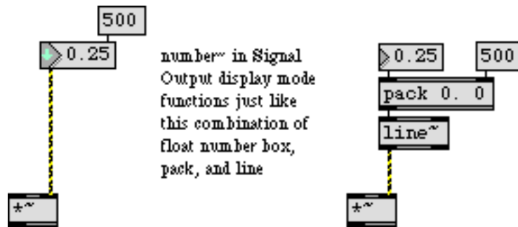
number~ can send a linear ramp signal from its old value to a new value
